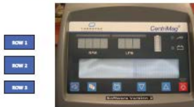
Primary Console Control Panel
